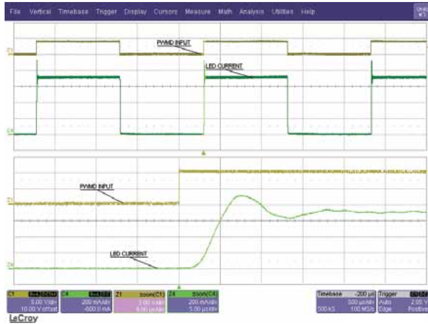
Fig. 3. PWM Dimming – Rising Edge Waveform
