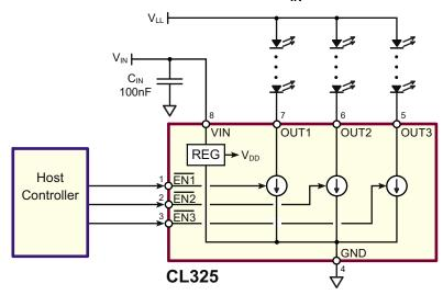
CL325 power dissipation may be lowered by supplying the CL325 from a voltage source ( $V_{IN}$ ) that is lower in voltage than the LED supply ( $V_{II}$ ).
